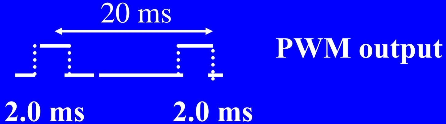
**Servo motor at +90° forward position**
