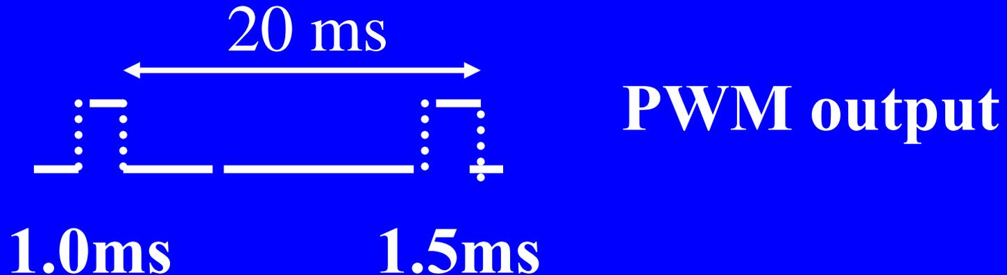
**Servo motor at  $-90^\circ$  reversed position**
