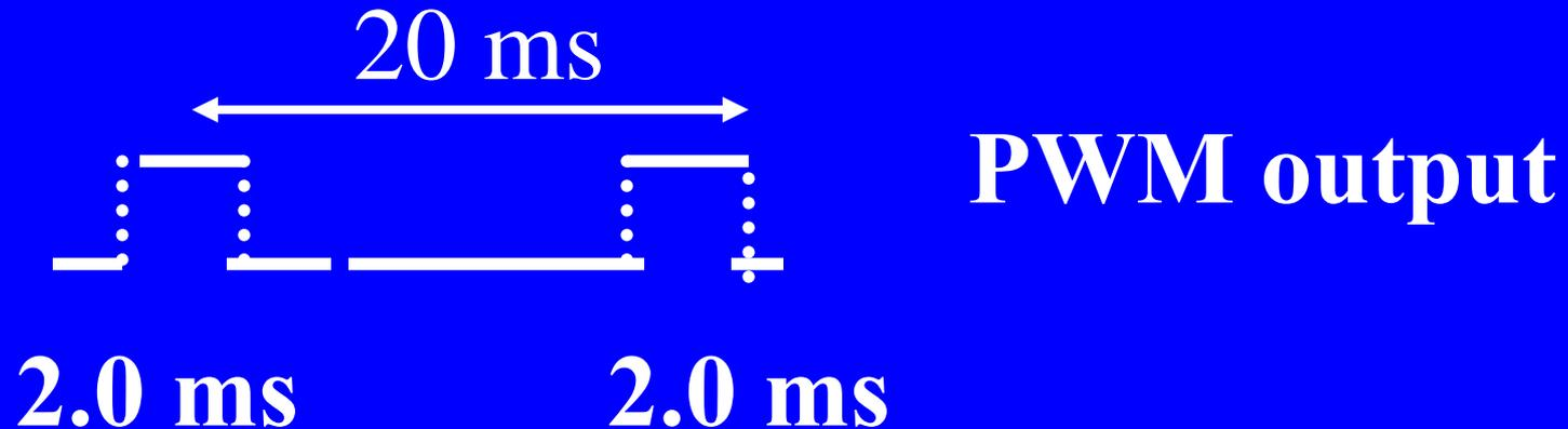
**Servomotor at +90° forward position**
