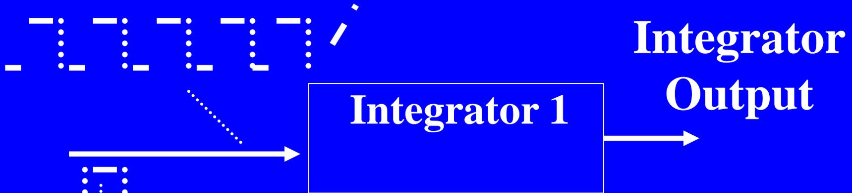
Analog output  $V \propto +[(2^n - x)]$  and T1 programmed between 1.0 ms to 2.0 ms
